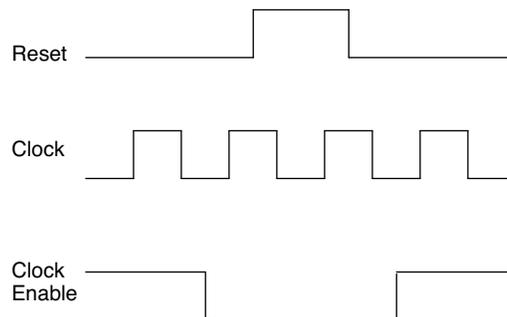
If all clock enables remain enabled, the EBR asynchronous reset or GSR may only be applied and released after the EBR read and write clock inputs are in a steady state condition for a minimum of  $1/f_{MAX}$  (EBR clock). The reset release must adhere to the EBR synchronous reset setup time before the next active read or write clock edge.
